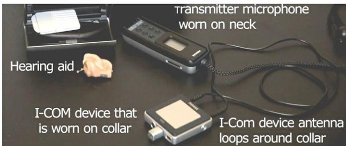
**Fig. 2.** Custom Phonak (Warrenville, IL) hearing aid (worn in the dog's ear) with wireless transmitter microphone (worn by dog owner) and I-COM receiver (worn on the dog's collar). Owner's voice can be transmitted up to 30 ft. (*Courtesy of* University of Cincinnati FETCH~LAB, Cincinnati, OH.)
