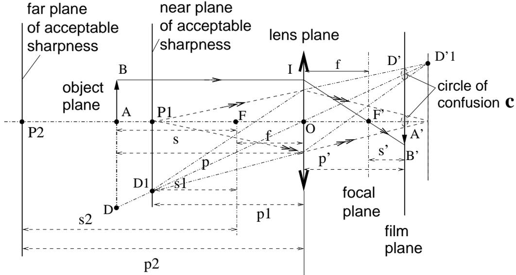
Figure 1: Depth-of-field distances  $s_1$ ,  $p_1$  and  $s_2$ ,  $p_2$  for a given circle of confusion  $c$
