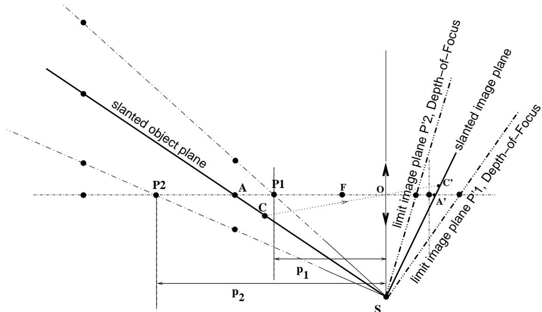
P1 and P'1 are optically conjugated through the camera lens of focal length  $f$  same for P2 and P'2, when  $H \gg f$ , and  $p \gg f$
