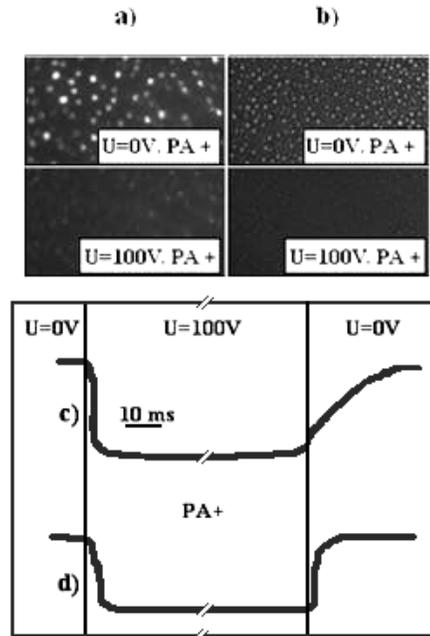
**Figure 6.** The microscopic images of LCE (8% ZhK1289 - silicon oil) in crossed polarizers without field and in electric field: droplet size about 20 μm (a) and about 10 μm (b); c) and d) – oscillograms corresponding to a) and b).
