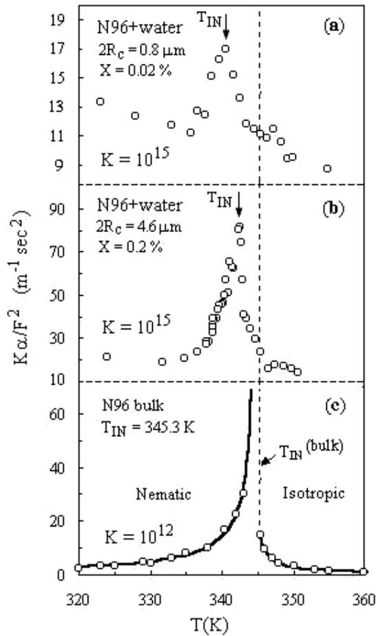
**Figure 2.** The temperature dependence of ultrasonic absorption ( $\alpha$ ) at frequency  $F=2.7$  MHz (points) for LCE samples with  $2R_c=0.8 \mu\text{m}$  (a) and  $2R_c=4.6 \mu\text{m}$  (b);  $K$  – dimensionless coefficient. The data for the bulk N96 reference sample are also shown in (c). Solid lines represent the power-law approximation.
