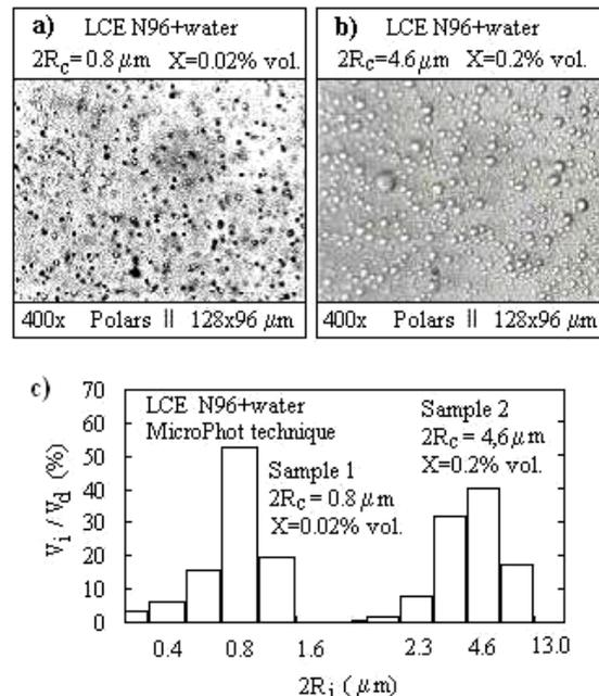
**Figure 1.** Microscopic images (a, b) of LCE samples with different average radius ( $R_c$ ) of droplets.  $X$  – concentration of LC in water; c) - the distribution of droplets on sizes in samples (a, b) obtained by micro-photometrical technique. The height of each column represents the volume  $V_i$  of liquid crystal per into total volume  $V_d$  of LC in emulsion for drops with sizes indicated on the horizontal axis  $R_i$ .
