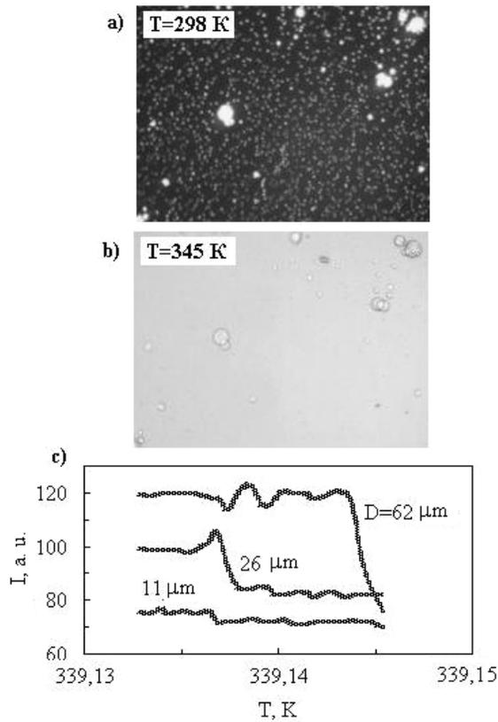
**Figure 5.** The microscopic images of LCE (ZhK440-silicon oil) at two temperatures: a) – nematic phase, crossed polarizers; b) – isotropic phase without polarizers; c) – brightness of light corresponding to droplets of different sizes.
