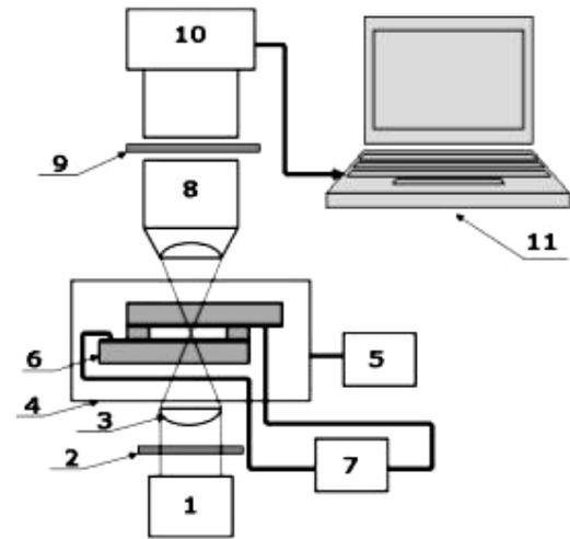
**Figure 3.** The block diagram of microscopic setup: 1 - source of light , 2 - polarizer, 3 - lens, 4 - thermostat, 5 - thermo regulator, 6 - acoustic-optical cell, 7 – low frequency generator 8 - objective of the microscope, 9 - analyzer, 10 - digital video camera, 11 - computer.
